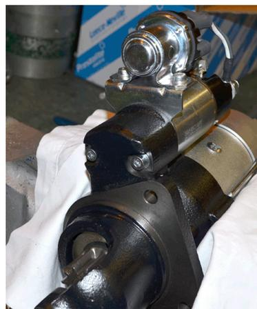
5. Tighten up the relay / solenoid lead connections (loosened in operation 1).
